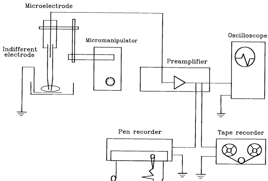
Fig. 1. Intracellular recording of gill epithelium equipment schematic.
