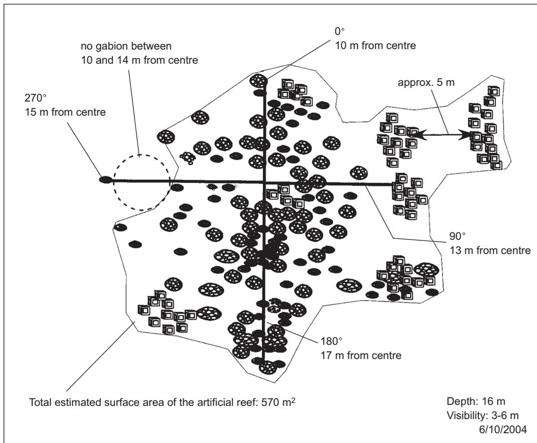
**Fig. 3.** Schematic diagram of artificial reef consist of 75 concrete cubes ( $75\text{ cm} \times 75\text{ cm} \times 75\text{ cm}$ , 170 kg) and 400 gabions (five to six natural stones, approx. 20 kg).
