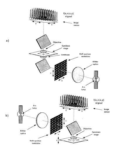
Fig.1. The EMCP optical setup. a) transmission configuration, b) epi-illumination configuration
