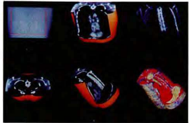
Fig. 2. Some 3D image processing techniques provided by the DISCOVER system. (a) The manipulation with a specified depth ( z = 145 ). (b) The volume surface rendering after the manipulation (a). (c) The volume rendering of the object (b). (d) Another manipulation with a specified depth ( z = 190 ). (e) The volume surface rendering after the manipulation (d). (f) The volume rendering of the object (e).
