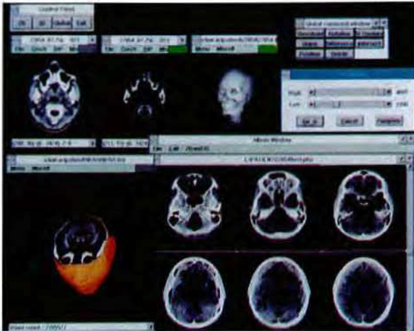
Fig. 1. The graphical user interface of the DISCOVER system. The global command window is on the upper-right corner. The album window is on the lower right corner. The 2D image and 3D image windows under "NCKU DISCOVER" are activated (see the green boxes) and are thresholded simultaneously.
