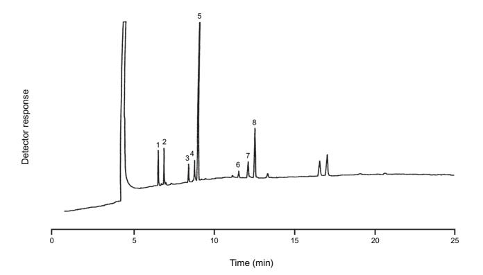
**Fig. 1.** Gas chromatogram of the combined wash of female crude extract. Gas chromatography was performed on a 30-m X 0.25-mm Carbowax 20 M column. The temperature was programmed to rise from 100 to 190 °C at 5 °C/ min. Identifications of peaks: (1) 12:Ac, (2) Z7-12:Ac, (3) 14:Ac, (4) Z7-14:Ac, (5) Z9-14:Ac, (6) 16:Ac, (7) Z7-16:Ac, and (8) Z11-16:Ac.
