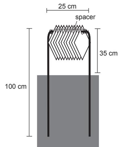
Fig. 2. Settlement racks used in the coral-recruitment study in southern Taiwan. Racks were set into the sediment (darker area).
